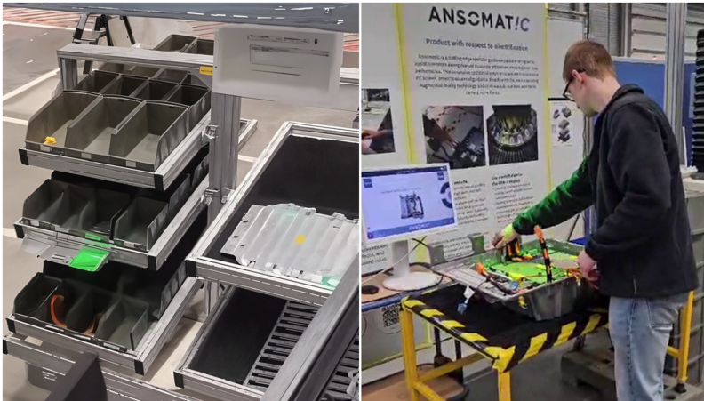
Figure 5. Pick-to-light projections of digital work instructions on the materials cart and on the assembly table. Source: Authors' own work
